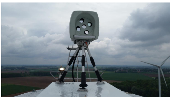
Figure 6.4 Leosphere 5 beam LiDAR mounted on top of SMV6
