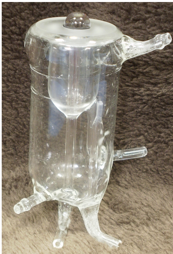
Figure 3.2: Photo of cell with hemisphere resting on o-ring (no clamps)
