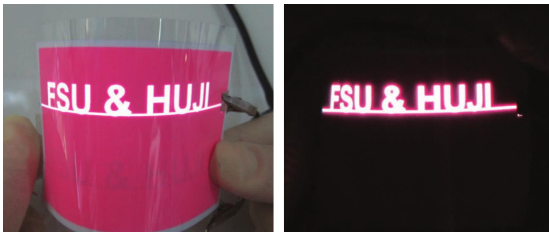
Figure 2.37: Electro luminescent printed electronic devices sintered using combined low pressure plasma and microwave flash sintering [68].
