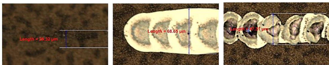
Figure 3.55: Increasing pulse energy of a P2 process on U1 CIGS with a larger spot, nominal size \sim 50 \mu\text{m} . There is no process which produces consistent acceptable results.
