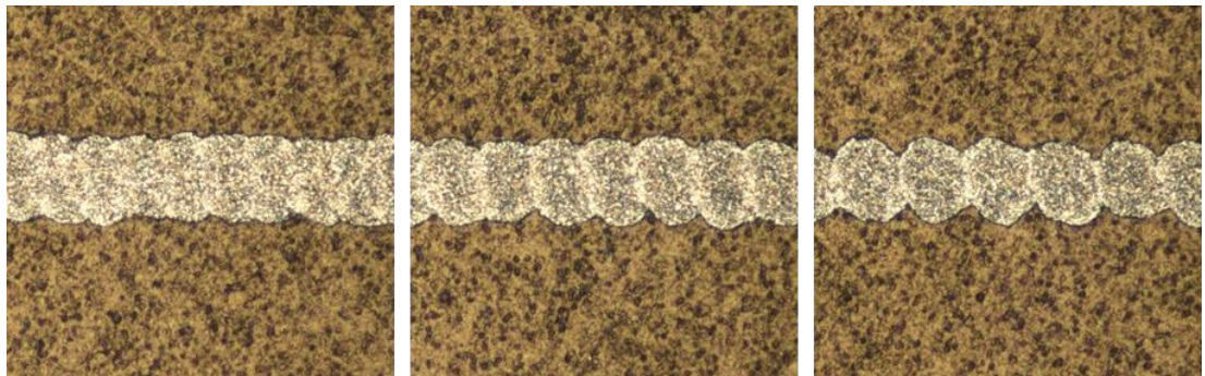
Figure 3.53: The effect of increasing beam translation velocity on the P3 process, in all cases the spot size is \sim 32\mu\text{m} . The beam speeds were 1.1, 1.4 and 1.7 m/s giving shot overlaps of \sim 35 , 20 and 5% respectively. This demonstrates that there is a robust process at a range of overlaps.
