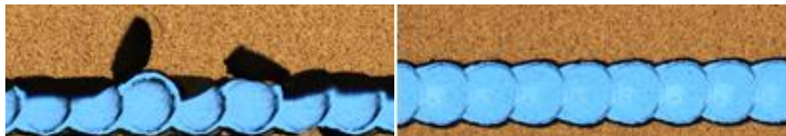
Figure 3.17: Circular mask imaging with the green laser incident through the glass. Left; Without the new sample handling procedures. Right; the new sample handling procedures increase layer adhesion and remove delamination when scribing.
