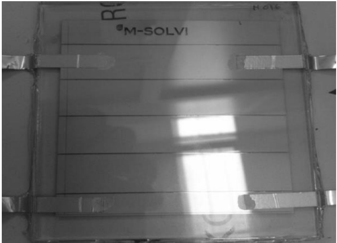
Figure 5.17: A mini-module encapsulated at M-Solv for damp heat testing. Two pieces of glass sandwich the active layers, a 1cm boarder has been laser edge deleted around the perimeter of the module to aid adhesion. 3M charge collection tape allows electrical connection.
