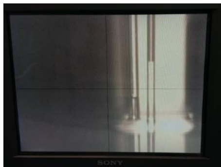
Figure 2.5. Picture of the liquid rise in the capillary tubes obtained with the setup based on the differential CR method for a mixture composed of CO 2 and n-decane.
