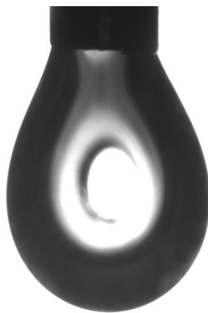
Figure 2.8. Example of a drop of water in a CO 2 atmosphere captured with the setup based on the PD method at P = 3.66 MPa and T = 333 K.
