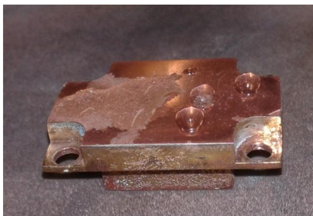
Figure 2.8: This shows a simple test to verify if a layer of SiO 2 has been deposited, where droplets of H 2 O appear to wet SiO 2 and clusters on Cu. The cloudy material on the left side of the sample is SiO 2 which has not stuck properly to the sample and would not be used in the UHV rig, however for the H 2 O test this will suffice.
