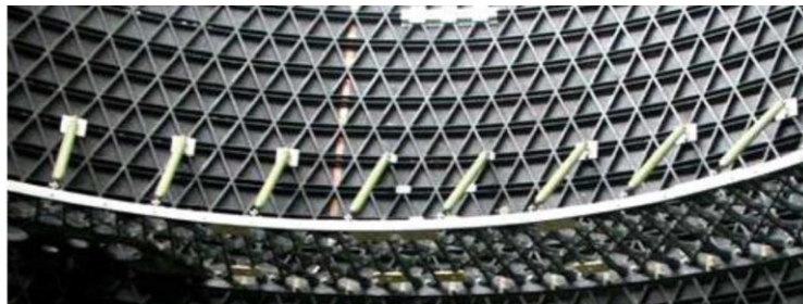
Figure 1 A barrel in a lattice structure developed for the rocket engineering application
