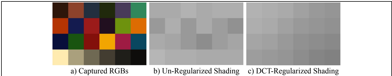
Figure 2: The shadings of the capture RGBs (a) are estimated by naïve ALS (b) and ALS with DCT smooth shading regularization (c).
