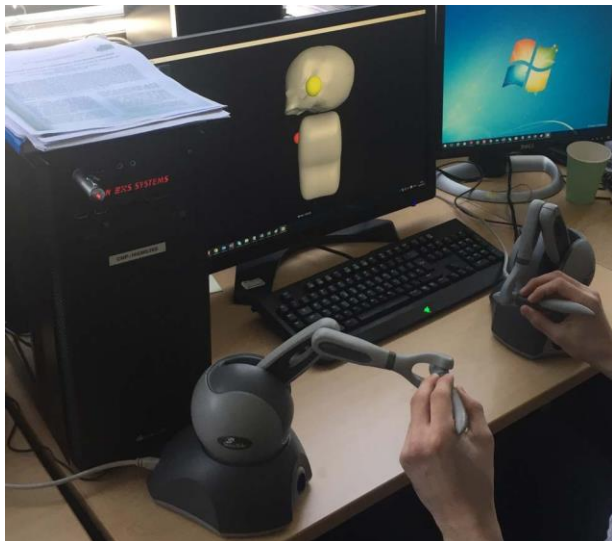
Figure 6. Figure 6. Experimental setup of the BirthViewHaptics software showing the GUI and the Phantom Omni haptics UI.
