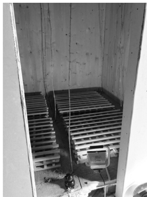
Fig. 1. View inside a typical compartment prior to ignition for configuration Alpha showing the four wooden cribs and gas phase thermocouple trees.
