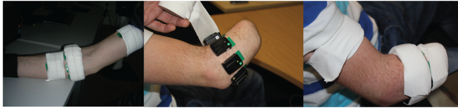
Fig. 2 Sensor placement. Eight EMG-IM sensors were equally spaced around the participants' forearm (3 cm below the elbow), two targeted the EDC and FDS muscles, and two were placed on the biceps and triceps muscles. Elastic bandage was used to keep sensors positions fixed. Sensor placement shown for an able-bodied ( left ) and an amputee subject ( centre, right )
