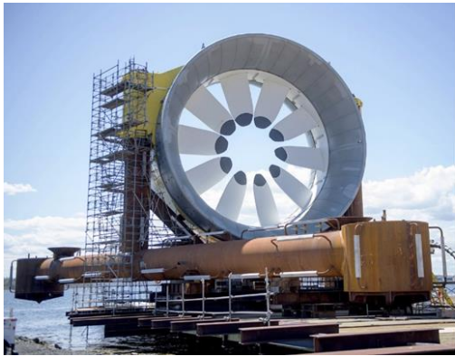
23 24 Figure 1-2 DCNS / OpenHydro 500 kW rated turbine (left, image credit: The Canadian Press) with installation at the Paimpol 25 Bréhat site, Northern France (right, image credit: DCNS)
