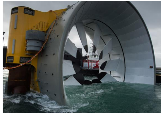
23 24 Figure 1-2 DCNS / OpenHydro 500 kW rated turbine (left, image credit: The Canadian Press) with installation at the Paimpol 25 Bréhat site, Northern France (right, image credit: DCNS)
