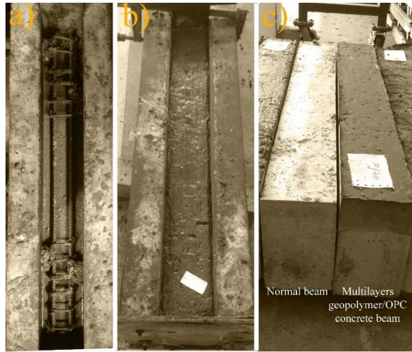
Fig. 3. Casting of different layers and final beam products.
