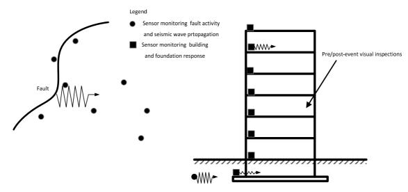
Figure 1: Collecting data via seismic monitoring and inspections.
