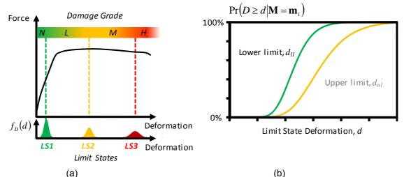
Figure 10: Definition of damage grades and corresponding limit states: a) force-deformation behaviour, and b) cumulative probability distributions  $P[D \ge d|\mathbf{M}=\mathbf{m}_i]$  of the limit state distributions conditional on model  $\mathbf{m}_i$ .
