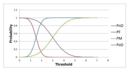
Figure 8: Variation of conditional probabilities PnD, PF, PM, PoD with threshold T.
