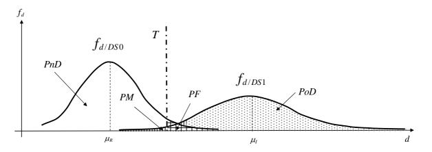
Figure 6: Distributions in the undamaged  $(f_{d/DS0})$  and in the damaged  $(f_{d/DS1})$  configurations
