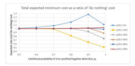
Figure 4: Comparison of total expected cost of decisions to use different monitoring systems for buildings with different prior seismic damage probabilities in Example 1.
