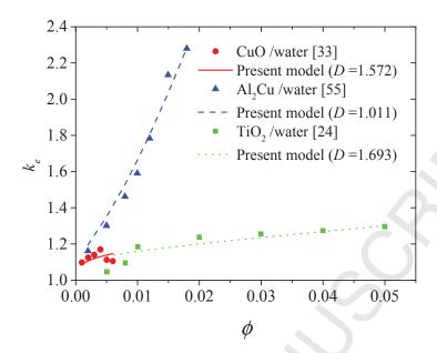
Fig. 2. Comparison between the total dimensionless effective thermal conductivity  $k_e$  from fractal model and experimental data in different concentration  $\phi$ .
