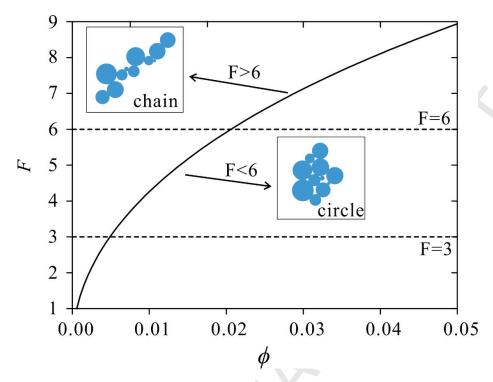
Figure 1. Relationship between F and concentration  $\phi$  in Eq. (11). The dashed line for F=3 and F=6 [34] representing respectively sphere and ellipse for suspended aggregation.
