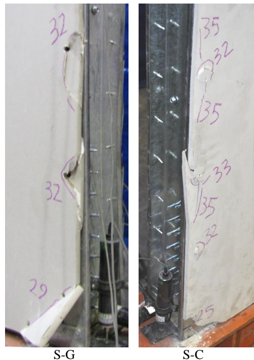
Fig. 10. Cladding fractures in region CD
