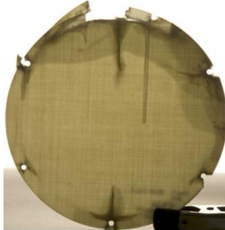
Fig. 18. Damaged test plate after the shock loading in CST [4].
