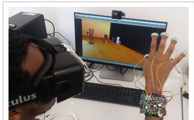
FIGURE 5 | Virtual reality setup with Oculus Rift and Leap Motion.
