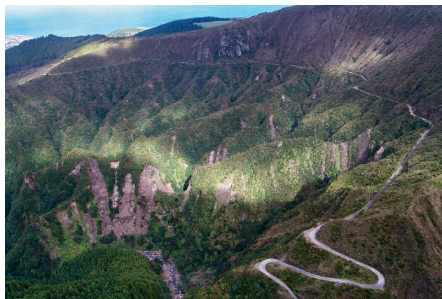
Fig. 3. Aerial view of Lombadas valley where the landslides associated scars triggered by the 2005 seismic swarms can be observed.
