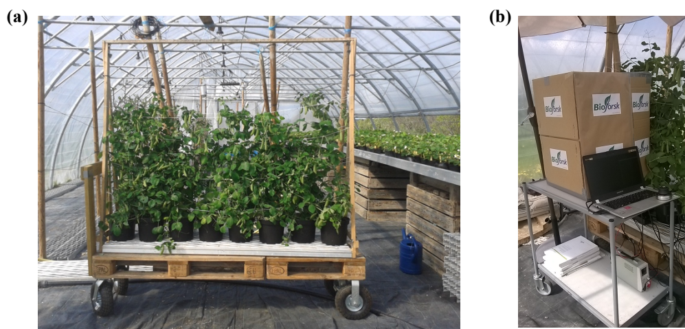
Fig. 5 Experimental setup at NIBIO Apelsvoll. (a) Sugar snap pea modular carrier inside the plastic greenhouse. (b) Moving desk carrying the partial shade and equipment (laptop, spacenavigator and power supply). The partial shade is covering the robot arm and its working environment
