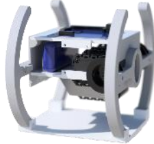
Fig. 3. 3D model of the servo mount section, displaying ribs either side, which attaches to the spine, servo mounting boards, servos, and underside servo brake and plate
