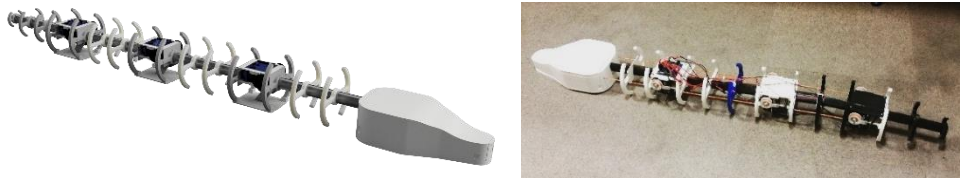
a) 3D rendering of the snake robot design. b) Basic working prototype of the snake robot.
