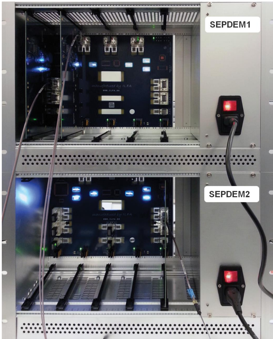
Figure 5-21: Two test and measurement platforms SEPDEM1 and SEPDEM2
