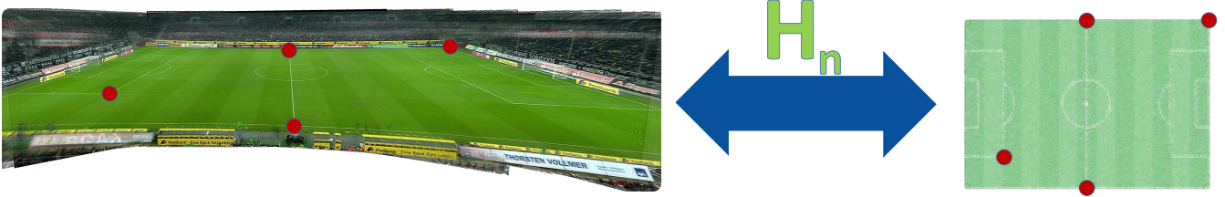
Fig. 3: The chosen points for the transformation of the panoramic (left) into the normalized (right) view must allow referencing distances in both directions of the main axes. Afterwards, a calculated homography H_n enables the transformation of panoramic view into normalized view and vice versa.
