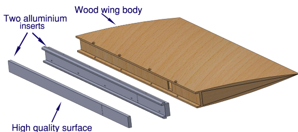
Figure 2: Model: swept wing with blunt leading edge. Overview of the design.
