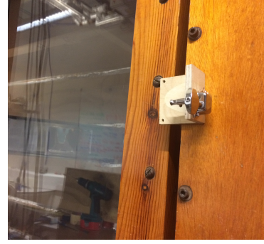
Figure 5: Mechanism to tighten the string upstream of the model
