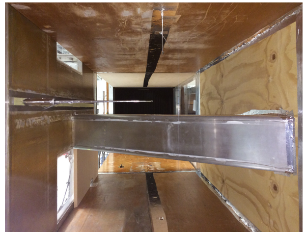
Figure 3: Blunt leading-edge wing mounted in the wind tunnel
