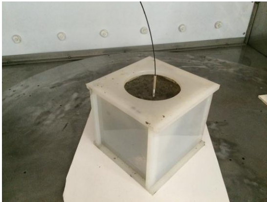
Fig. 9 Photo of 150 mm concrete cube cast in PP mould in microwave
