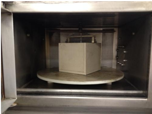
Fig. 4 Photo of 100 mm concrete cube cast in PEEK mould in microwave
