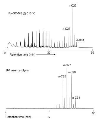
Figure 1: *M/z* 57 chromatograms for a solvent extracted kerogen isolate of higher plant material from the late Cretaceous Period, ~70 Ma (KT Boundary, Brownie Butte, Montana). The top chromatogram shows the *m/z* trace for the sample analysed by conventional Pyroprobe pyrolysis at 610°C. The bottom *m/z* trace is for the same sample analysed by LA at 213 nm.
