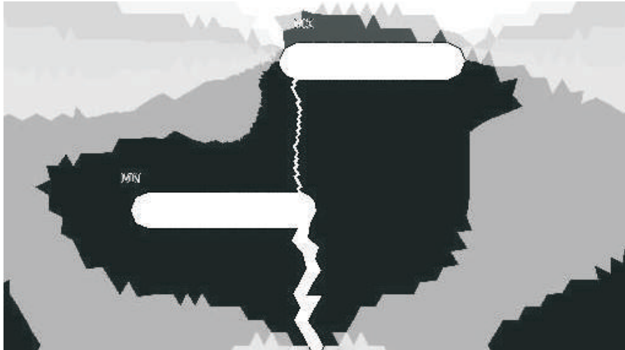
Figure 10 Distribution of reduced stresses according to Huber's hypothesis in the model obtained by means of the finite element method
