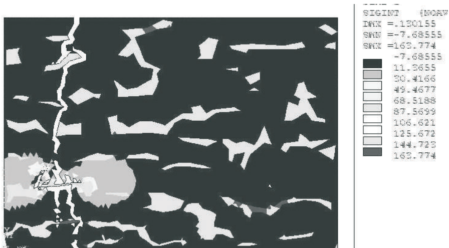
Figure 6 Distribution of reduced stresses according to Huber's hypothesis in the model studied using the metallographic method obtained by means of the finite element method
