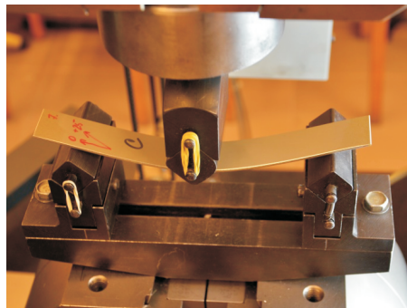
Figure 7 FML specimen during three point bending test
