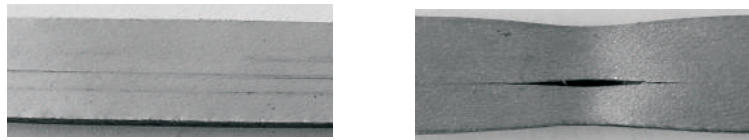
Figure 1 Metallographic specimen of a sheet with visible inclusions
