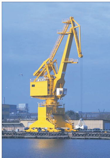
Figure 1 Harbor jib crane
