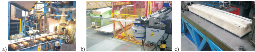
Figure 1 Aluminium profile: extrusion (a), bending (b) and stretching (c) (A. Mróz photo)
