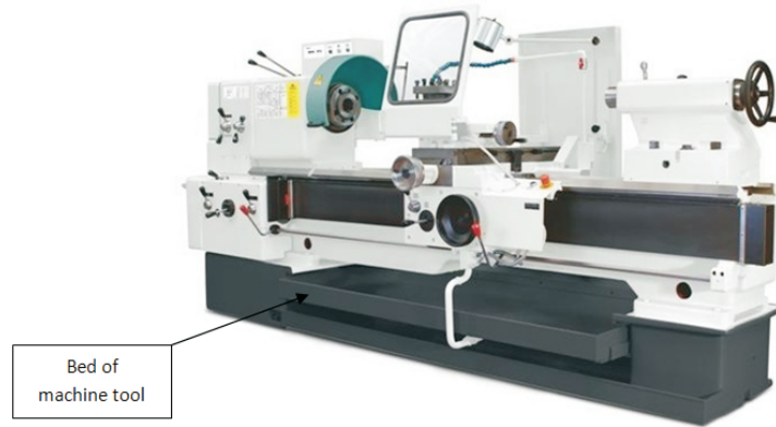
Figure 2 Centre lathe with marked bed of machine tool
