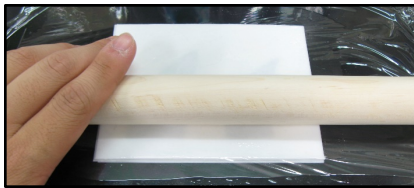
PVDF-leaf sandwich between two layers of filter is pressed with a rolling pin
