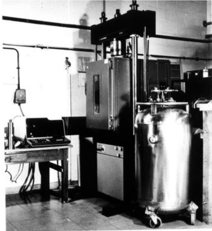
Figure 3.5 Instron testing machine fitted with the environmental chamber.
