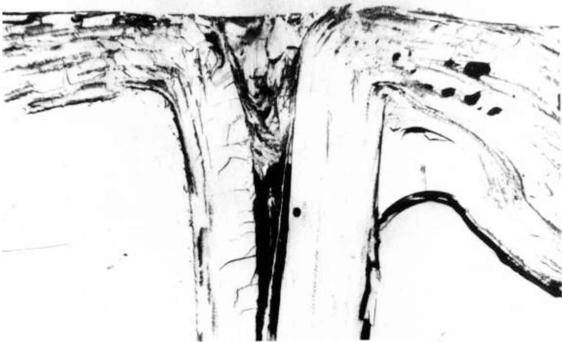
Figure 6.24 Section through the crush zone of a glass mat-polyester tube crushed at room temperature.
