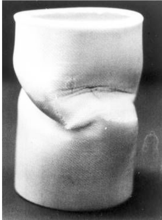
Figure 6.30 Macro photograph of a Tufnol tube crushed at 110 °C showing the buckling mode.
