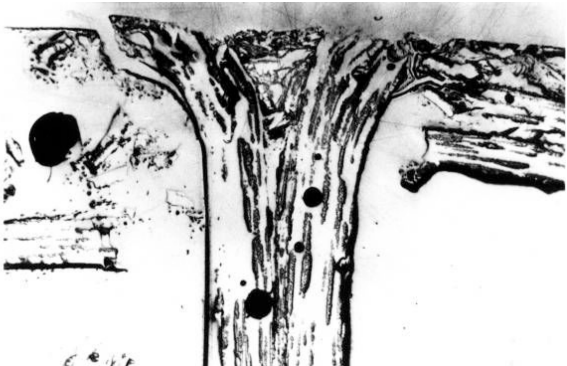
Figure 6.25 Section through the crush zone of a glass mat-polyester tube crushed at room temperature.
