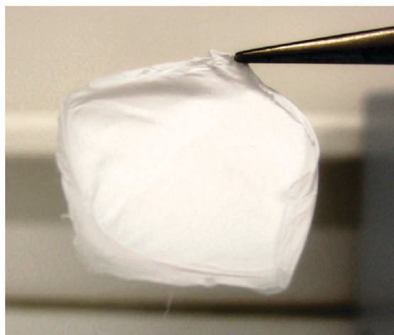
Fig. 3 Digital photograph of a non-woven ZIF-8-PVP fiber mat. The diameter is ca. 1.5 cm.
