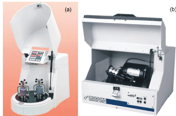
Fig. 2 (a) A high-energy ball mill “Pulverisette 7” (Fritsch, Idar-Oberstein, Germany) of the planetary type and (b) a SPEX 8000M shaker mill (Spex CertiPrep Inc., USA) of the vibratory type, often used nowadays for the mechanochemical preparation of nanopowders.
