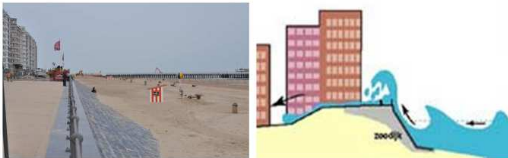
Figure 1. Typical promenade at the Belgian coastline (left) and the situation during storm (right).
