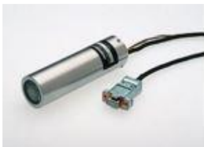
Figure 2.9 PMT: An integrated PMT module incorporating PMT detector, high-voltage supply, and photon counting circuitry. The PMT is vertically housed above of the flow cell to observe the light from the chemiluminescence reaction inside a box. The PMT module provides count linearity within a range of \pm 1\% at 20 \times 10^6 \text{ s}^{-1} which is able to be controlled directly by an external computer through an RS-232 interface.
