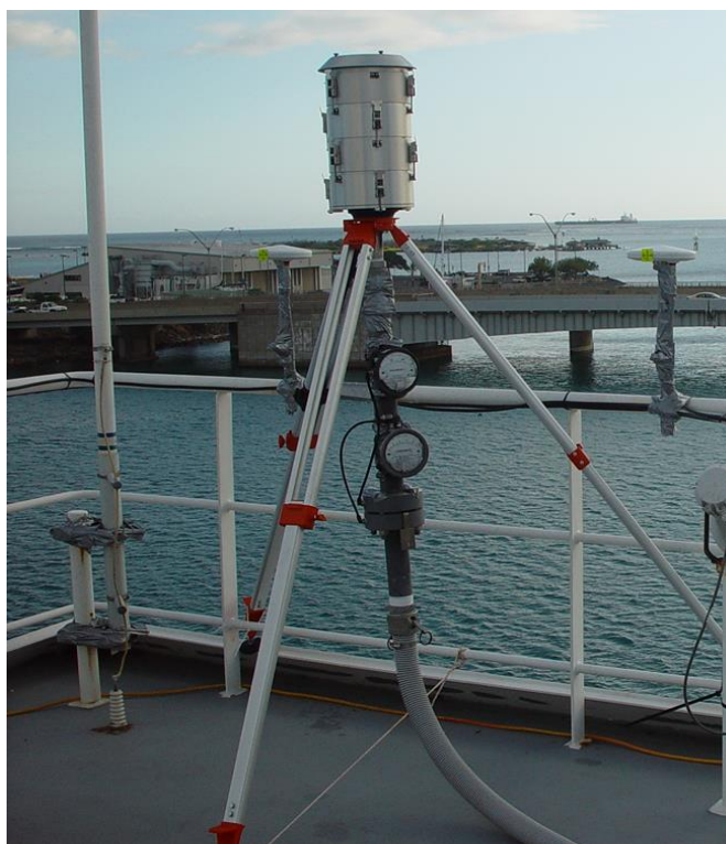
Figure 2.2 High-volume collector with regulated pump.
