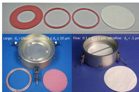
Figure 2.3 Four impactation and filtration substrates: large, coarse, fine and ultrafine (white filter).
