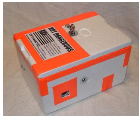
Figure 2: Styrofoam cooler modified for weather balloon launch.
