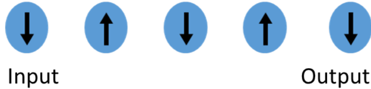
Figure 1.5: Bennett clocking using dipole coupled nanomagnetic logic.
