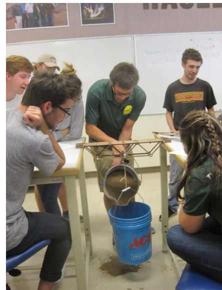
Figure 10: Students assemble truss structures prepared from digital fabrication equipment and test them to failure in Activity #6
