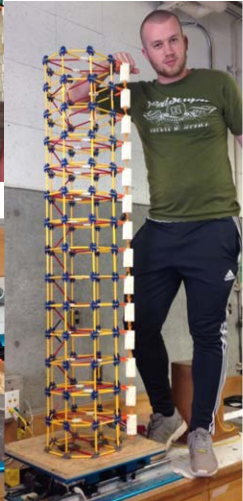
The 14 story building is ready to shake
