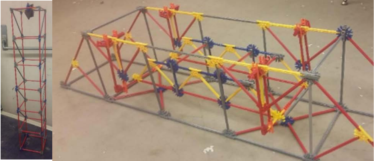
Figure 9: The six story building (left) and the base isolator system (right) to which the building is attached
