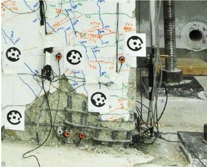
(a) Dowel action of the BE bars
