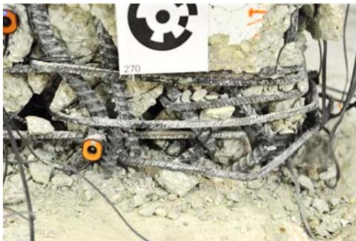
Figure 13: Examples of confinement failure (Brueggen 2009)
