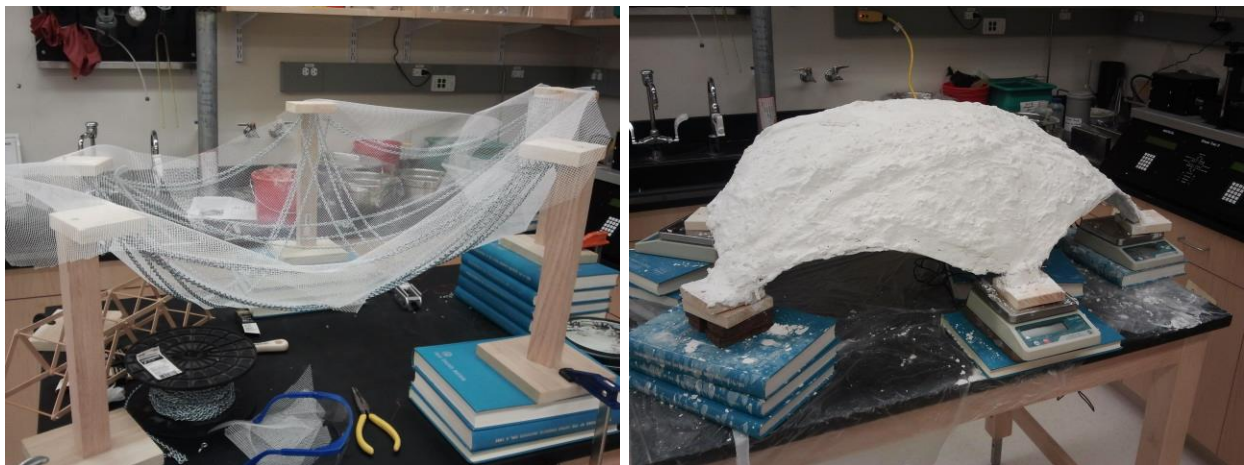
Figure 5. Thin-shelled Reinforced Concrete Dome Project: (Left) Hanging Mass Structure, (Right) Finished Dome Structure
