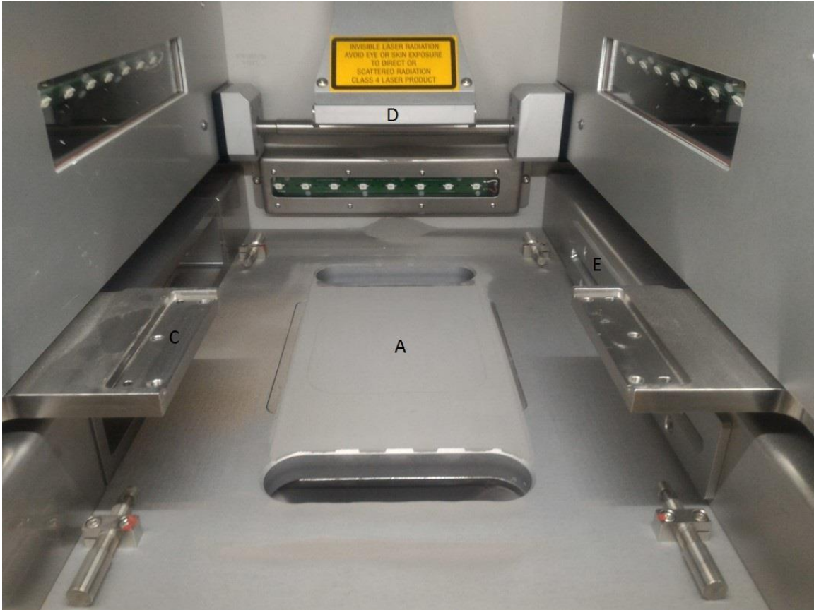
Figure 1. The SLM 125 HL build chamber. A) The build plate and elevator. C) Recoater Carriage. D) Power chute. E) Air flow vents.
