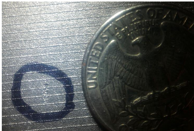
Figure 28. Bubble-forming scratch on the circular wall of Part #4.
