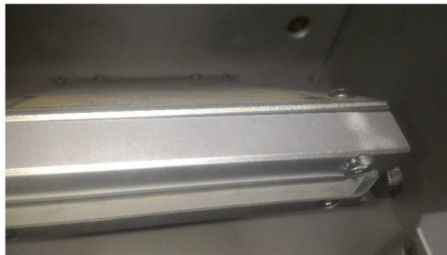
Figure 2. Stick-out of the front-right side powder gate screw that resulted in the obstruction of recoater motion.
