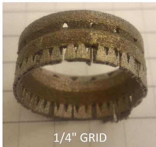
Figure 49. As-printed 4-chamfer ring. Upper triangle channels, while poor in geometrical resolution, are unobstructed their entire length.
