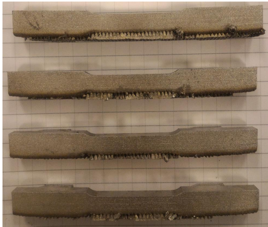
Figure 8. Warped modified tensile bars with burn-in and degradation along the downward facing surface.
