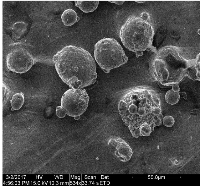
Figure 12. SEM image of particles adhered to the surface of the vertical wall of PAC-A-1.
