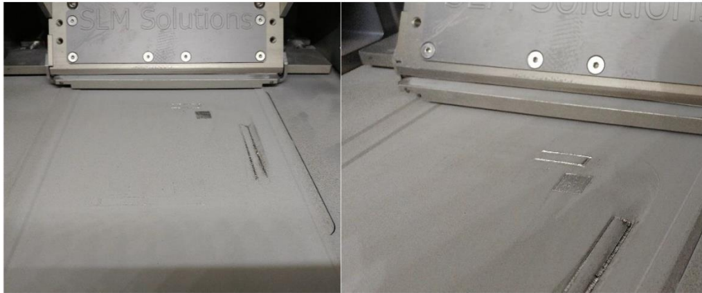
Figure 2. Poor powder coverage on the right side of the plate, affecting the right-side FullScale_QuarterCircle_NoLattice, the far-right rear Tensile Oversized V3, and the right-side of the rear FullScale_QuarterCircle_NoLattice.
