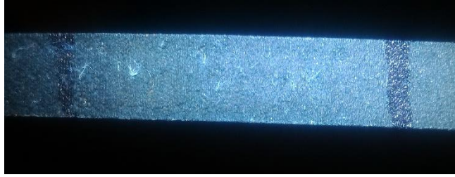
Figure 27. Location of bubble formation on Part #4. The surface lacks any visual indication of defects in the form of through-thickness channels.
