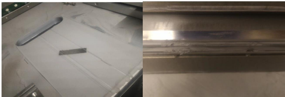
Figure 2. Powder bed tracks and the corresponding damaged recoater blade.
