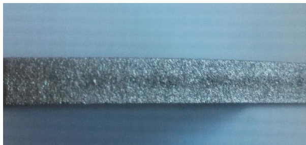
Figure 26. Mid-width dark coarsening on the upper cylindrical wall of Part #1.
