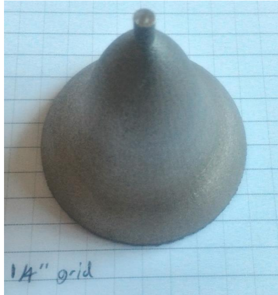
Figure 42. As-printed bell. Minor polygonization from the .stl to .slm conversion process is visible on the surface of the outer bell.
