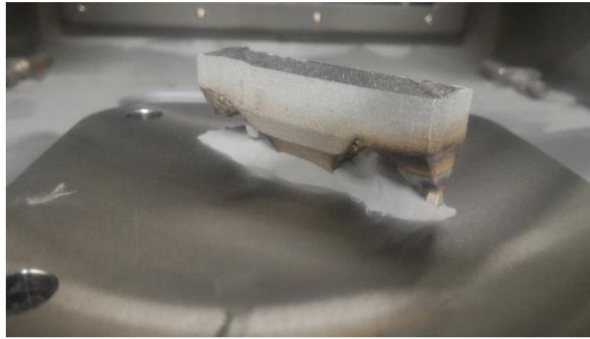
Figure 3. As-printed h_15 component with failed outer legs and burn-in characteristic of poor dimensional stability.
