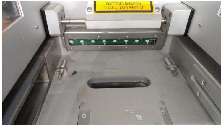
Figure 3. Left-side powder gate cam screw resting at the rear of the build chamber as discovered after removing the recoater.
