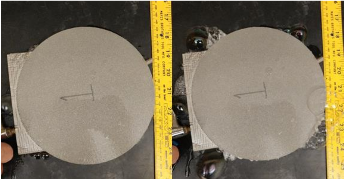
Figure 25. Soap-covered Disk #1 before and after air-pump induced internal pressurization.
