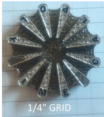
Figure 69. Top-down view of an IME Radial Card Holder Memento printed on the right-side of the build plate.
