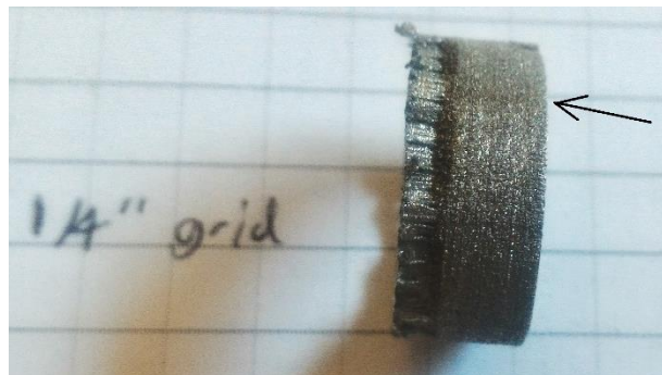
Figure 46. Dark bands on the outer wall of the Astrology ring.
