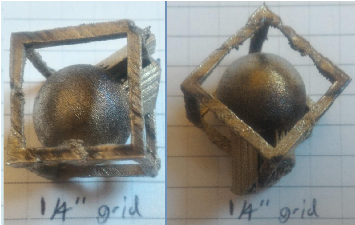
Figure 60. As-printed Cube with Caged Sphere. The effect of poor dimensional resolution caused by early damage to the recoater is exhibited by the cube members.
