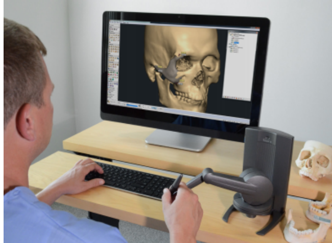
Figure 5. Geomagic Touch (PHANTOM) haptic stylus device being used in combination with visual simulation [18].
