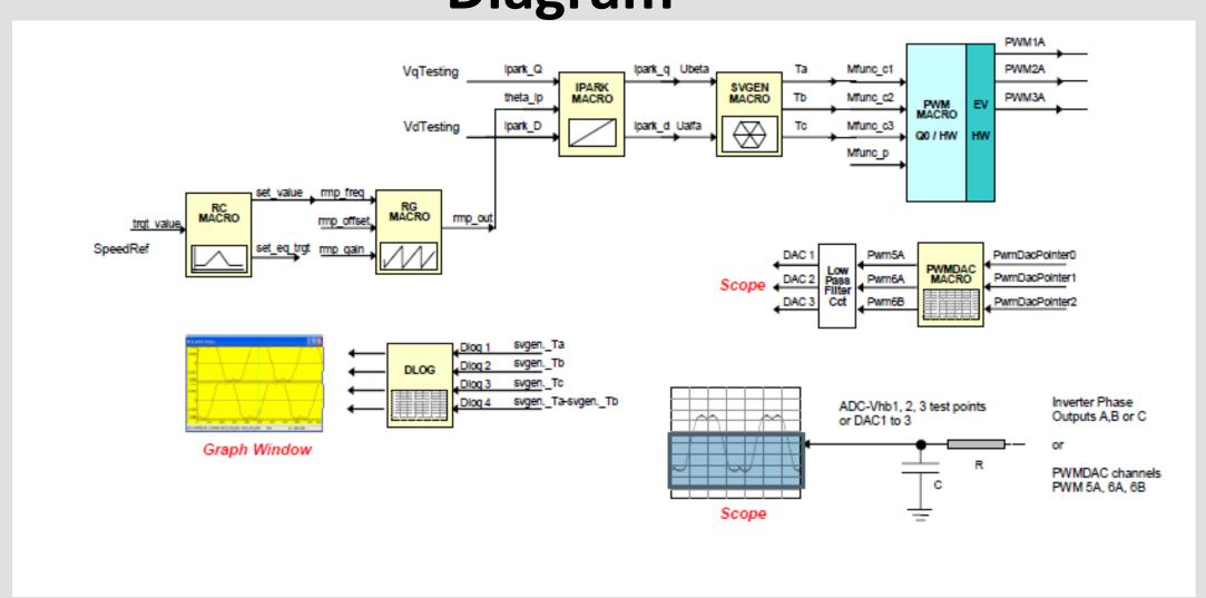
In this step the motor is disconnected and peak to peak measurements are taken.
