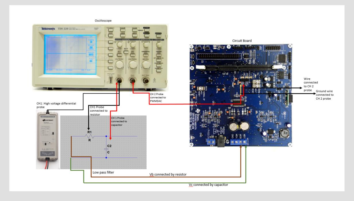
The diagram displays the actual setup of the first level experiment where the motor is disconnected. CH 1 is the voltage probe (10:1 ratio) connected to low pass filter, and CH 2 is connected to the PWMDAC pins on the circuit board.
