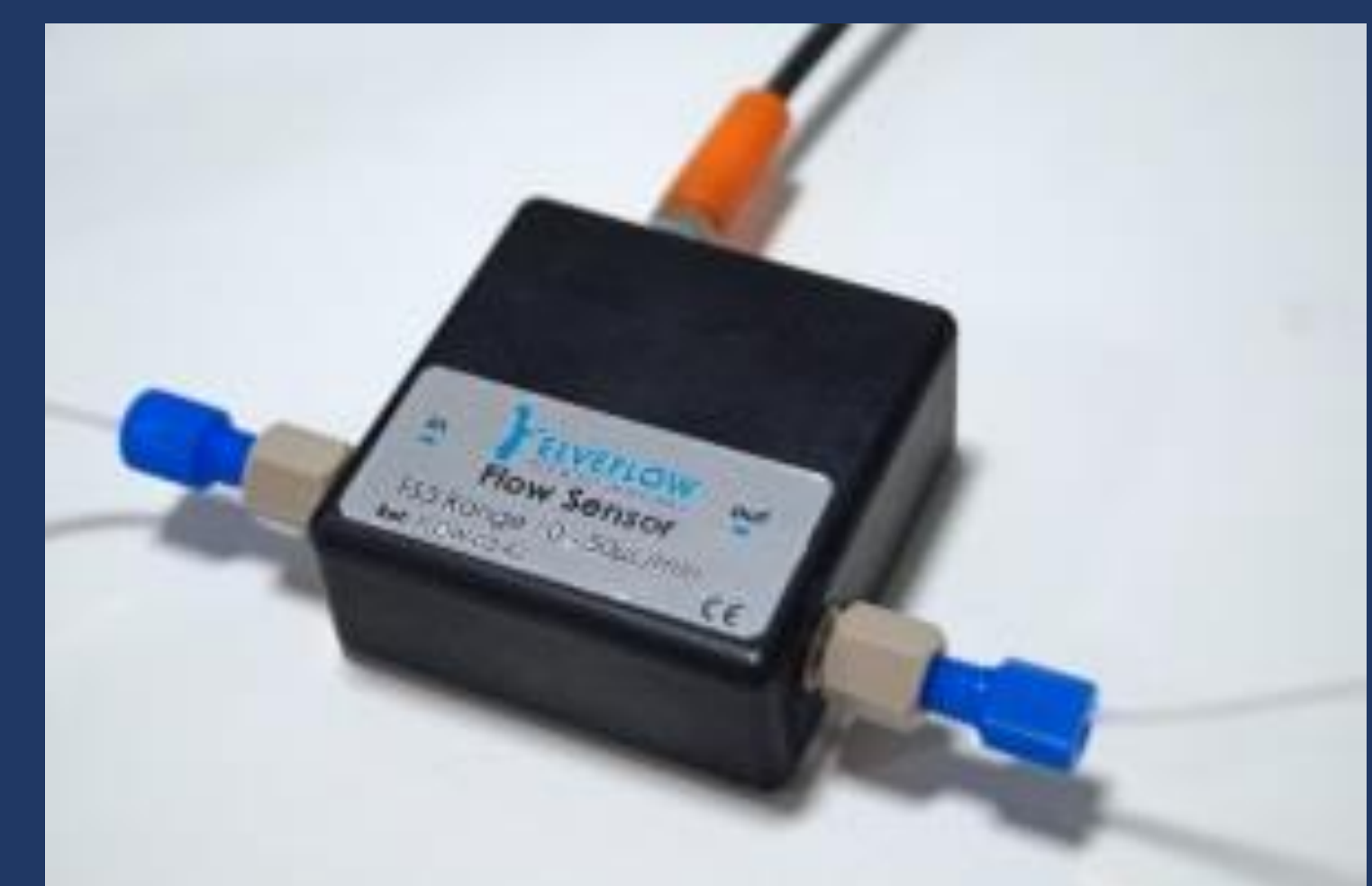
Figure 2: The flow sensors used come from Elveflow and have varied flowrate ranges.
