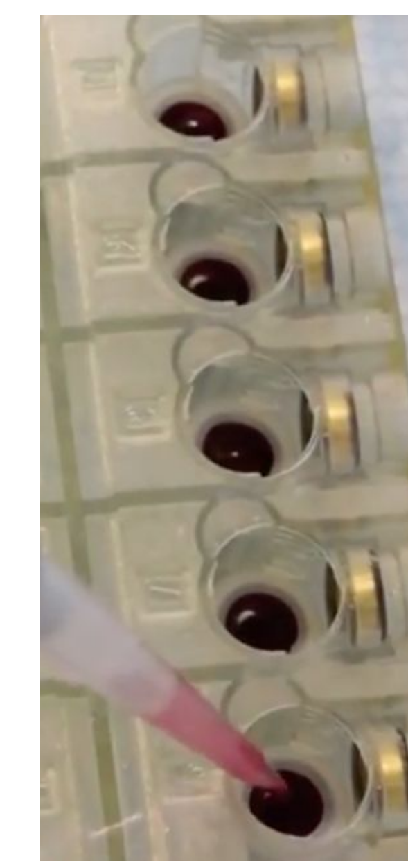
Figure 6: ICP wells filled with a colored agarose solution.
