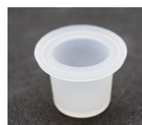
Figure 2: The silicon liner for the ICP wells. Referred to as the "well cup".
