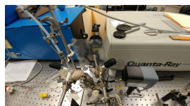
Figure 8. LIBS setup showing the laser, focusing lens, Pyrex cell, and the emission collection box.
