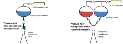
Figure 1. Diagram of a monopropellant thruster and a bipropellant thruster.
