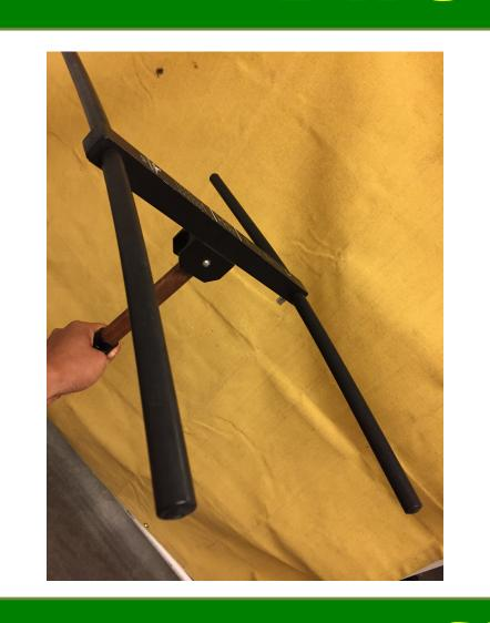
The directional "H" antenna has the better performance than typical handheld 3 element antennas used in the early days of telemetry. The result is better range performance and a more consistent pattern for location work.
