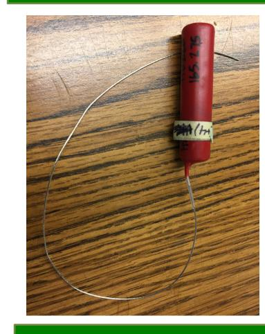
radio implant transmitters in fishers. weight is 11 grams. The standard life is 18 months.
