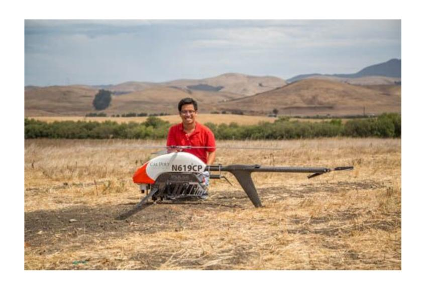
The **Pulse VAPOR55** is an electric Unmanned Aerial Vehicle (UAV). It is capable of automatic flight using pre-programmed mission instructions. The Pulse VAPOR55 can carry customizable payloads of up to 24 lbs, and it can operate at altitudes up to 10,000 feet and can cruise at 25 mph. It is designed for VTOL (vertical take-off and landing) operations.
